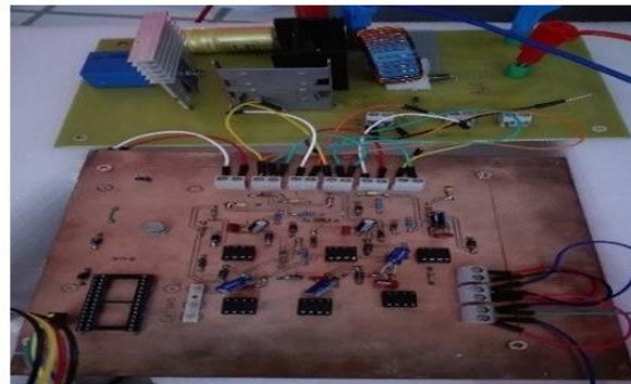
Fig. 10: Hardware set-up of the boost converter with the galvanic-isolation circuit.
